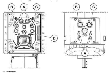
Value **Position Connection Description** Number Air hose with outer diamet-Α Air Max. 6 bar 4 er 4 mm, 2 pcs Air hose with outer diameter 6 mm, 2 pcs C1 8 wires i В Customer power/signal 30 V, 1.5 A C2 С Customer power/signal 30 V, 1 A or 1 Gbits/s 8 wires or ethernet Exhaust portii Φ10, 7~9L/min iii D ΕP
