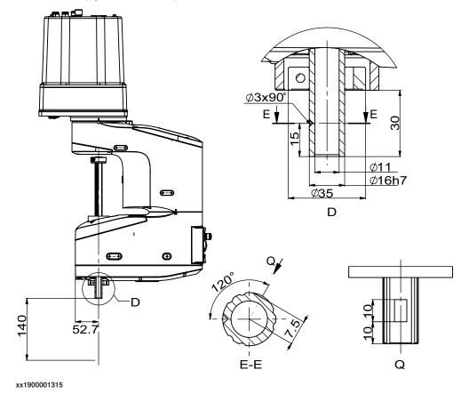
3.3.7 Fitting equipment on the robot (robot dimensions)
